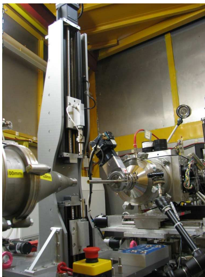
Fig. 21. Measuring system enabling tensile drawing of samples with simultaneous register of small-angle X-ray scattering patterns (synchrotron, Hasylab, Hamburg, Germany).
