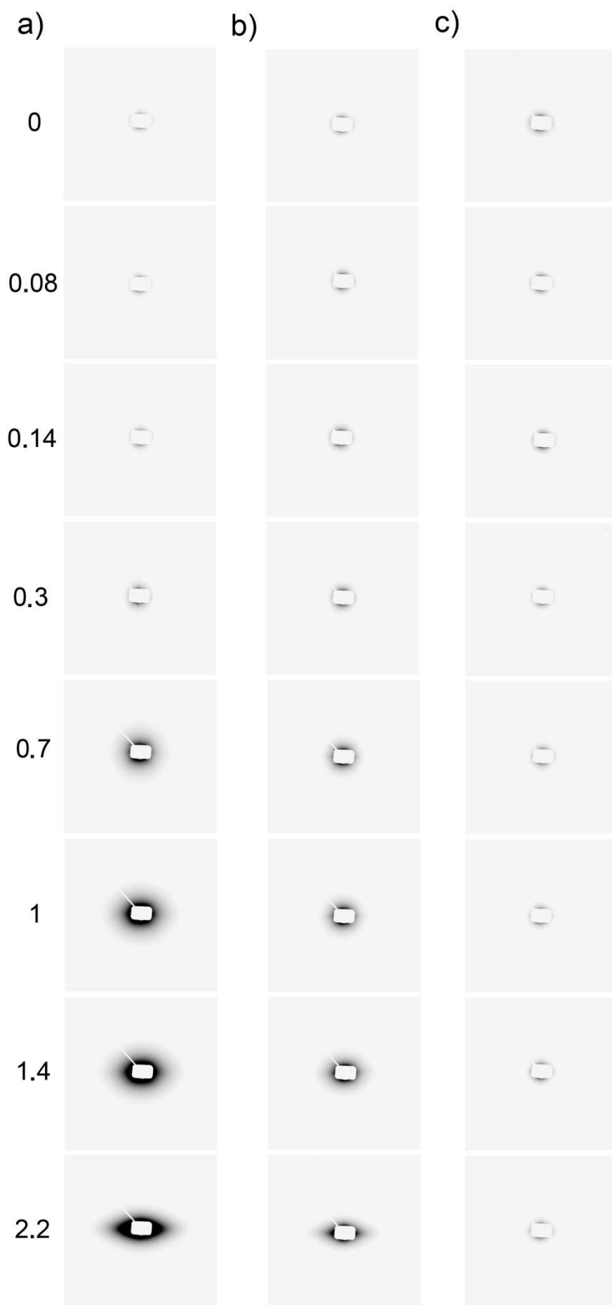
Fig. 70. Diffractograms of small-angle X-ray scattering of a series of samples of different water content: a) DS; b) MS; c) WS. Figures correspond to local strain of samples. Direction of deformation – vertical.
