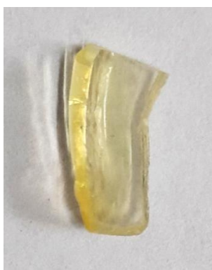
Figure S4. Photograph of the piece of PLA-TPE_EP/PAN network, sample II (the weight increase by 430 %).
